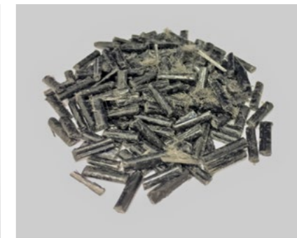
Good glass fiber impregnation after coffee mill test
