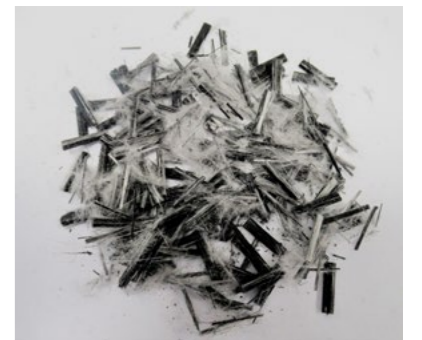
Poor glass fiber impregnation after coffee mill test
